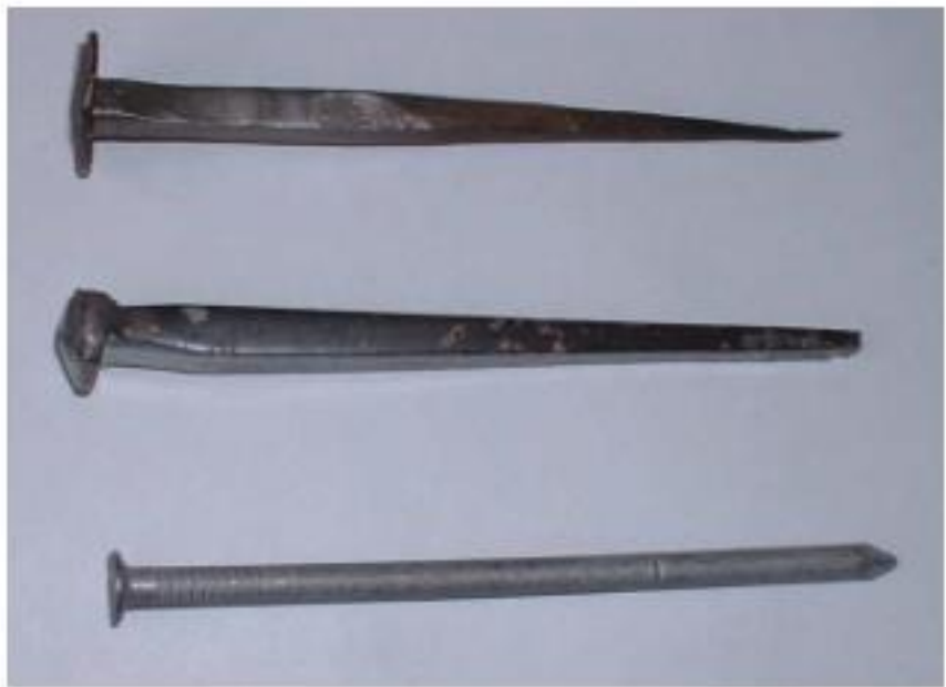
Three types of nails: wrought (top), cut (center), wire (bottom) (Glasgow Steel Company 2014).
